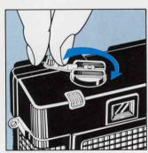
2. Then, flip open the film rewind crank and turn it in the direction of the arrow, printed on its handle (clockwise), until it turns freely. You will actually feel a change in the lever tension when the film is completely rewound into its cassette.
