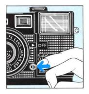
1. Push the flash operating button in the direction of the arrow (toward the lens). The flash will "pop-up" into place and automatically turn itself on.
