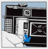
3. When the crank turns freely the film has been rewound into the cassette. Open the camera's back cover to remove the film, and have it processed. If you open the back cover before completely rewinding the film, you will ruin the pictures you have just taken on the film that has not been rewound into the cassette.
